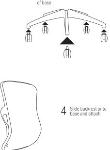
Insert castors into underside
